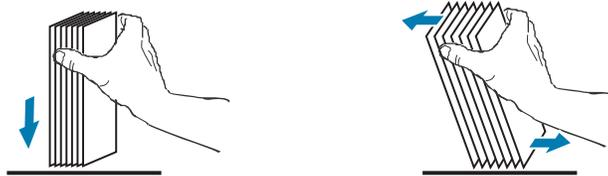
**Step 3.** Push the stack back and forth to an angle of about 45° from vertical, so as to separate all of the cards.
