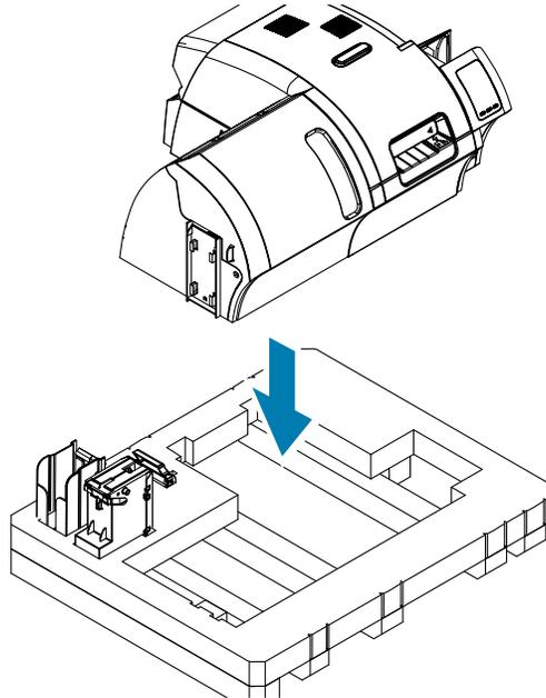
**Step 15.** Place the two corner blocks on top of the right front and left front corners of the lower foam insert.
