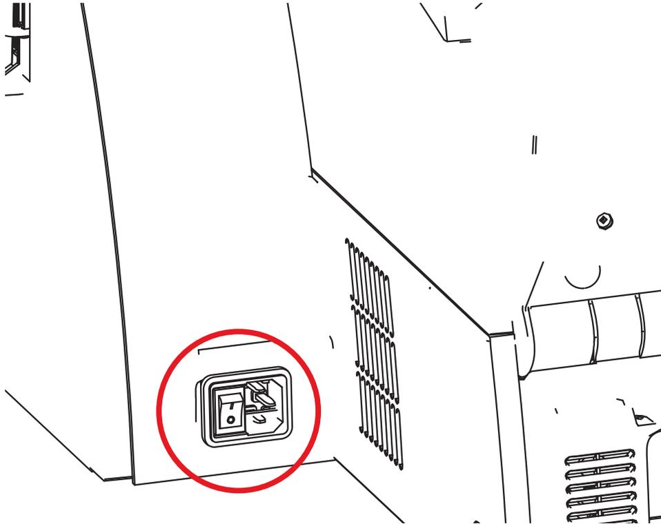
Press the upper portion of the power switch to the ON ( | ) position.
