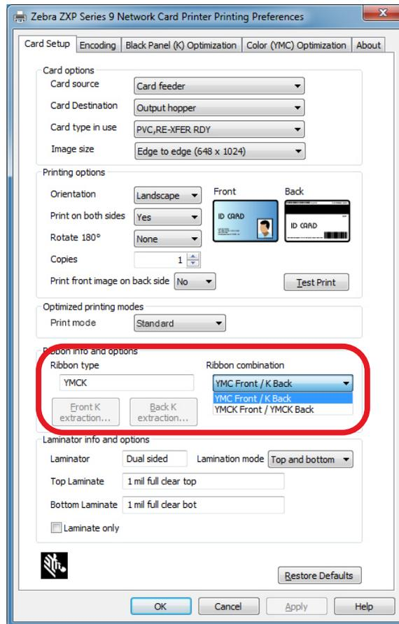
In the example above, the available ribbon combinations for the installed YMCK ribbon are YMC on the front of the card, and K on the back of the card; or YMCK on both the front and the back of the card. The available Ribbon combinations is also dependent on if printing is set to single- or double sided.
