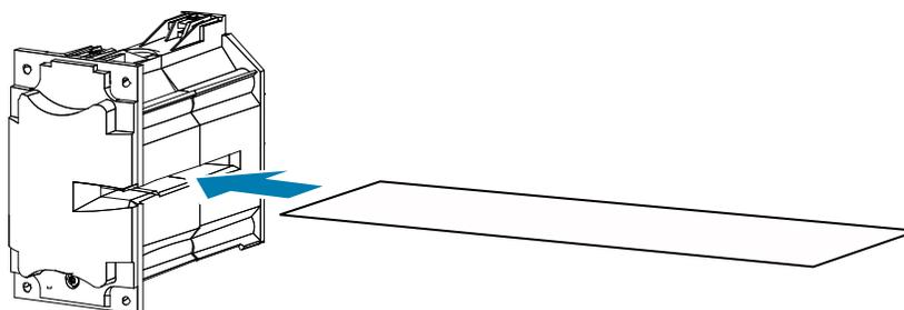
**Step 8.** Pull the card all the way through the heater assembly thereby cleaning the heater rollers.
