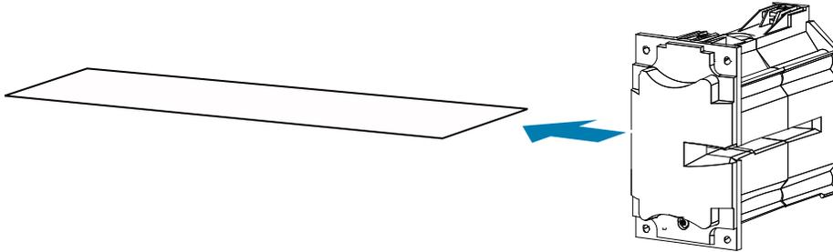
**Step 10.** Turn the card over, adhesive side up; and repeat Step 8, Step 9, and Step 10.
