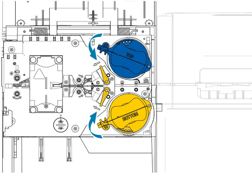
**Step 4.** Continue to turn the cassette. The locking lever will move to the left as the cassette rotates over the locking mechanism, and will then click into the locked (green) position.
