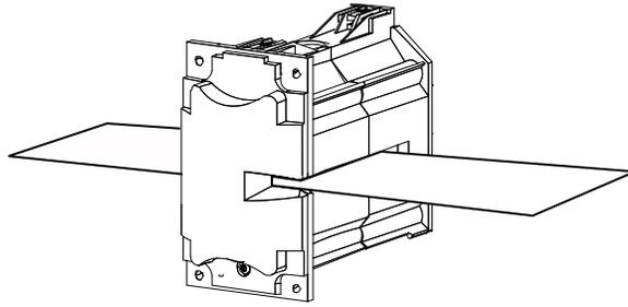
**Step 9.** Remove the card from the heater assembly.
