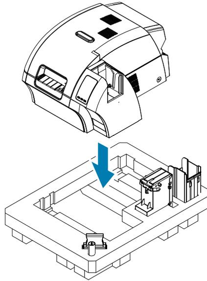
**Step 12.** Place the upper foam insert onto the printer, and gently press it down so it makes a snug fit on the printer—the top of the upper foam insert should be even with the upper edge of the shipping carton.
