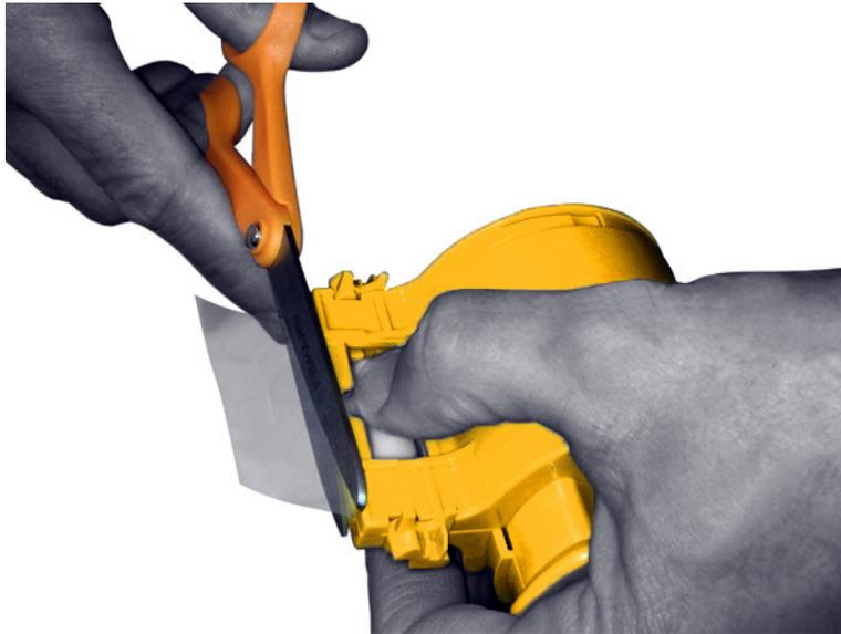
**Step 9.** Rotate the core to adjust the laminate overhang. Stop when the end of the laminate is just beyond the lip of the cassette, as shown below.
