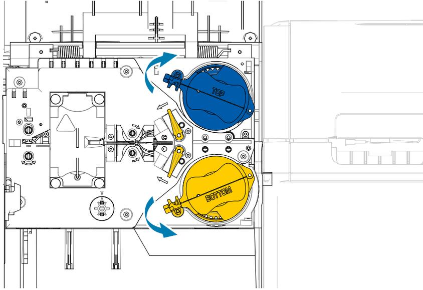
**Step 4.** Remove each cassette by pulling straight out from its spindle.
