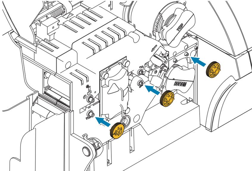
In some cases, a card may get wrapped around the laminator heater assembly rollers. In this case, the laminator heater assembly can be removed.
