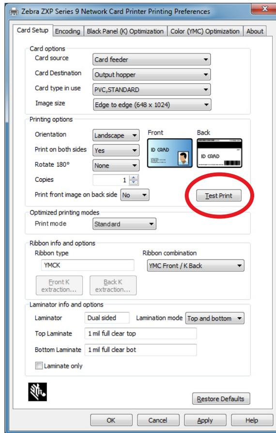
An enhanced test print feature is also available from the ZXP Toolbox. This feature offers a wider range of test cards to showcase the quality of print from the ZXP Series 9. The test card is printed according to the settings in the Card Setup tab.
