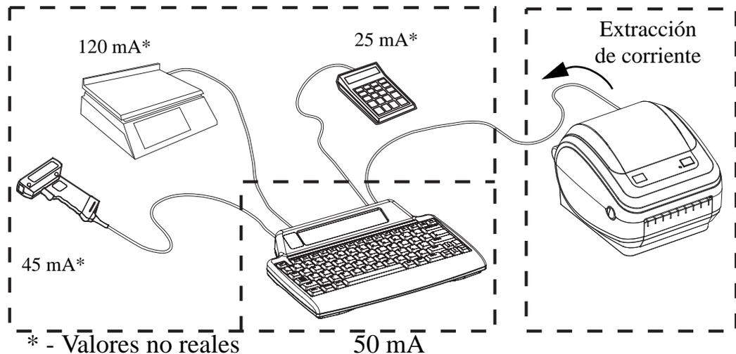
$$(45 \text{ mA} + 120 \text{ mA} + 25 \text{ mA}) + 50 \text{ mA} < \text{Corriente máx.}$$
