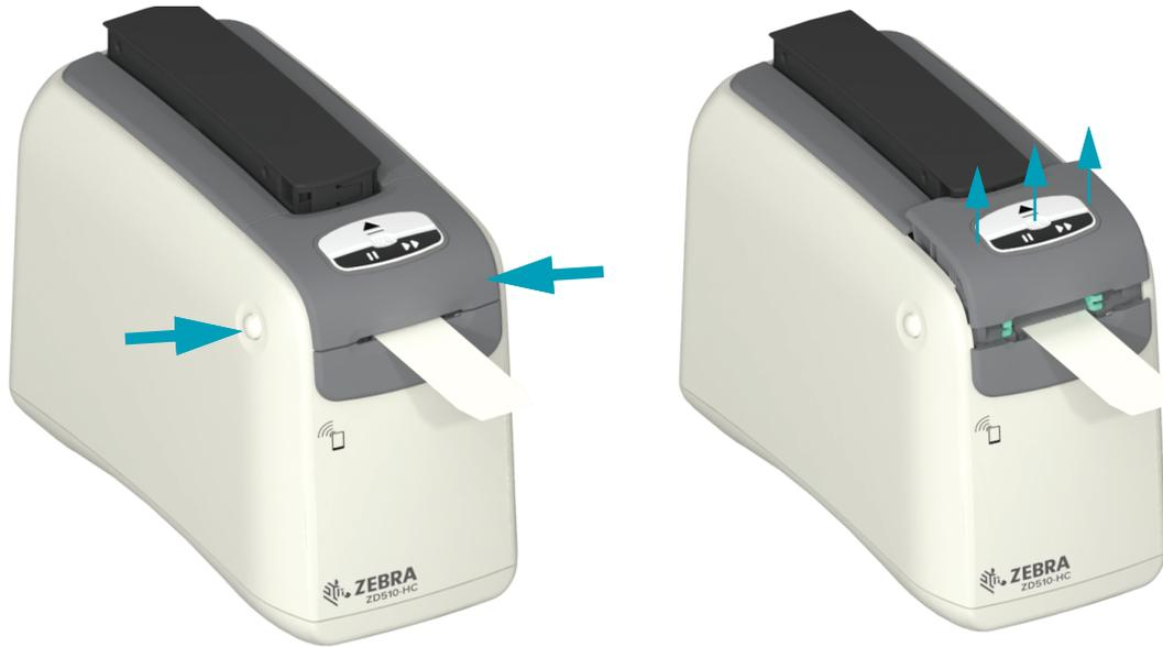
6. Lift the media cartridge out of the printer.
