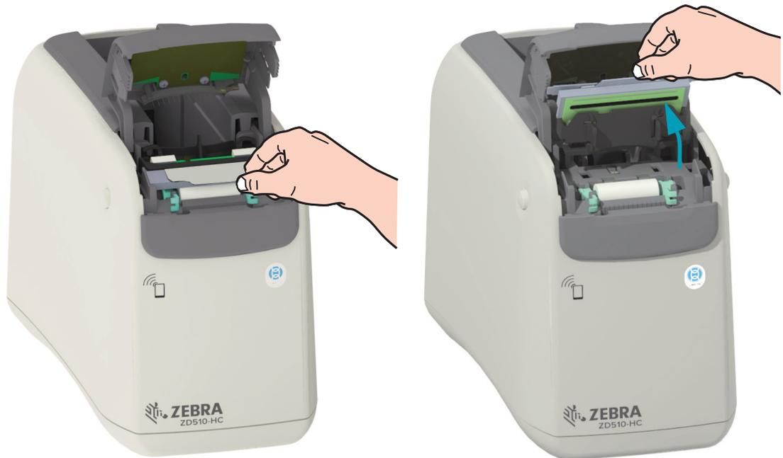
4. Rotate and lift the two (2) green arms on each side of the platen roller straight up. Holding the two (2) arms lift the Platen Roller Assembly out of the printer.
