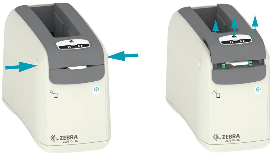
2. **Partially Opened** — The printer is ready at this stage for removing the media cartridge with media or packaging material.
