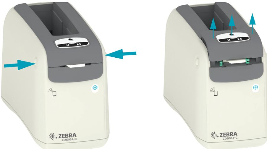
2. Lift the Upper Cover up until it stops and tilt the Upper Cover back for better access. The media path, printhead, platen roller and media sensor are now accessible.
