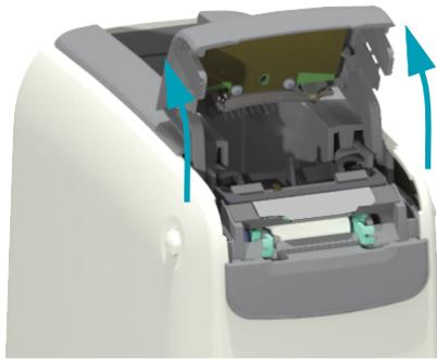
3. Lift the shiny aluminum metal tab on top of the Printhead assembly and lift it up. Lift the Printhead Assembly out and off the printer below it using the tab.
