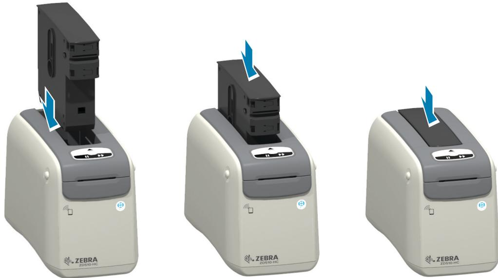
4. **Observe** - The printer prepares a wristband for printing, moves the media (wristband) to the Media Exit Slot (Ready to Print position), and reads the media cartridge's operating parameters and data.
