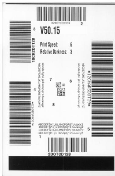
4. See Figure 17 and Table 18. Inspect the test labels and determine which one has the best print quality for your application. If you have a bar code verifier, use it to measure bars/spaces and calculate the print contrast. If you do not have a bar code verifier, use your eyes or the system scanner to choose the optimal darkness setting based on the labels printed in this self test.
