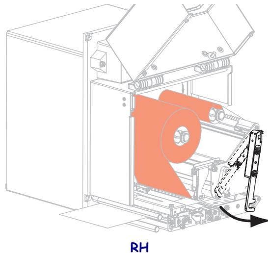
15. Raise the peel roller latch so that the peel roller assembly pivots downward.
