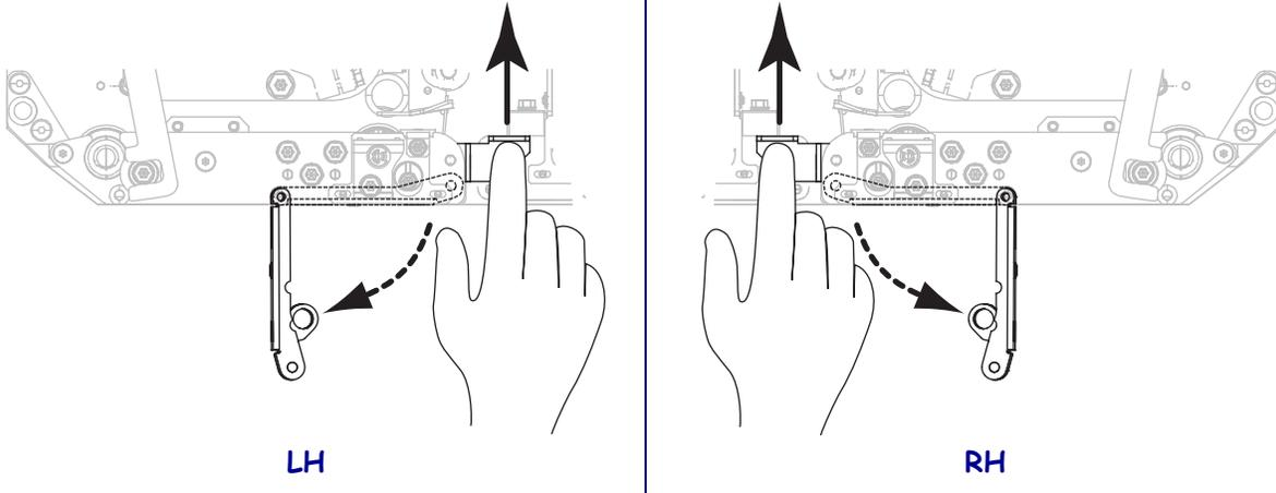
16. Thread the liner around the peel bar, under the platen roller, and through the peel roller assembly.
