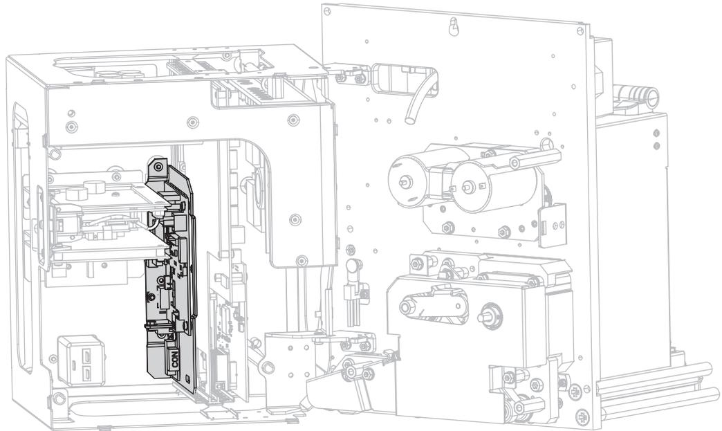
9. Disconnect the connectors (1) along the accessible edge of the applicator interface board. Note how the connectors are attached to assist with reattachment later in this procedure.
