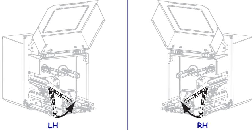
3. Extend approximately 8 in. (203 mm) of media past the peel bar. Remove and discard the labels from the liner on this exposed media.
