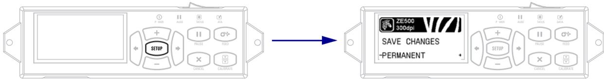
1. While in Setup Mode, press **SETUP** to exit the operating parameters. The LCD displays **SAVE CHANGES**.
