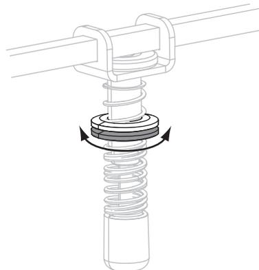
6. To lock the toggle pressure, tighten the locking nut against the adjusting nut.
