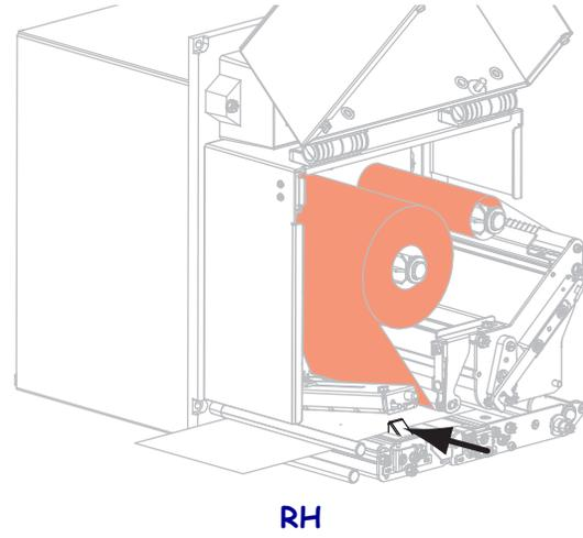
13. Press down on the pinch roller assembly until it locks closed.
