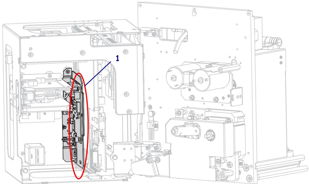
10. Gently pull the applicator interface board partially away from the back plane of the print engine.
