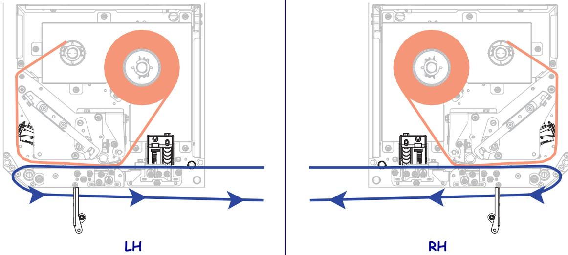
17. Rotate the peel roller assembly up until it locks into the closed position.
