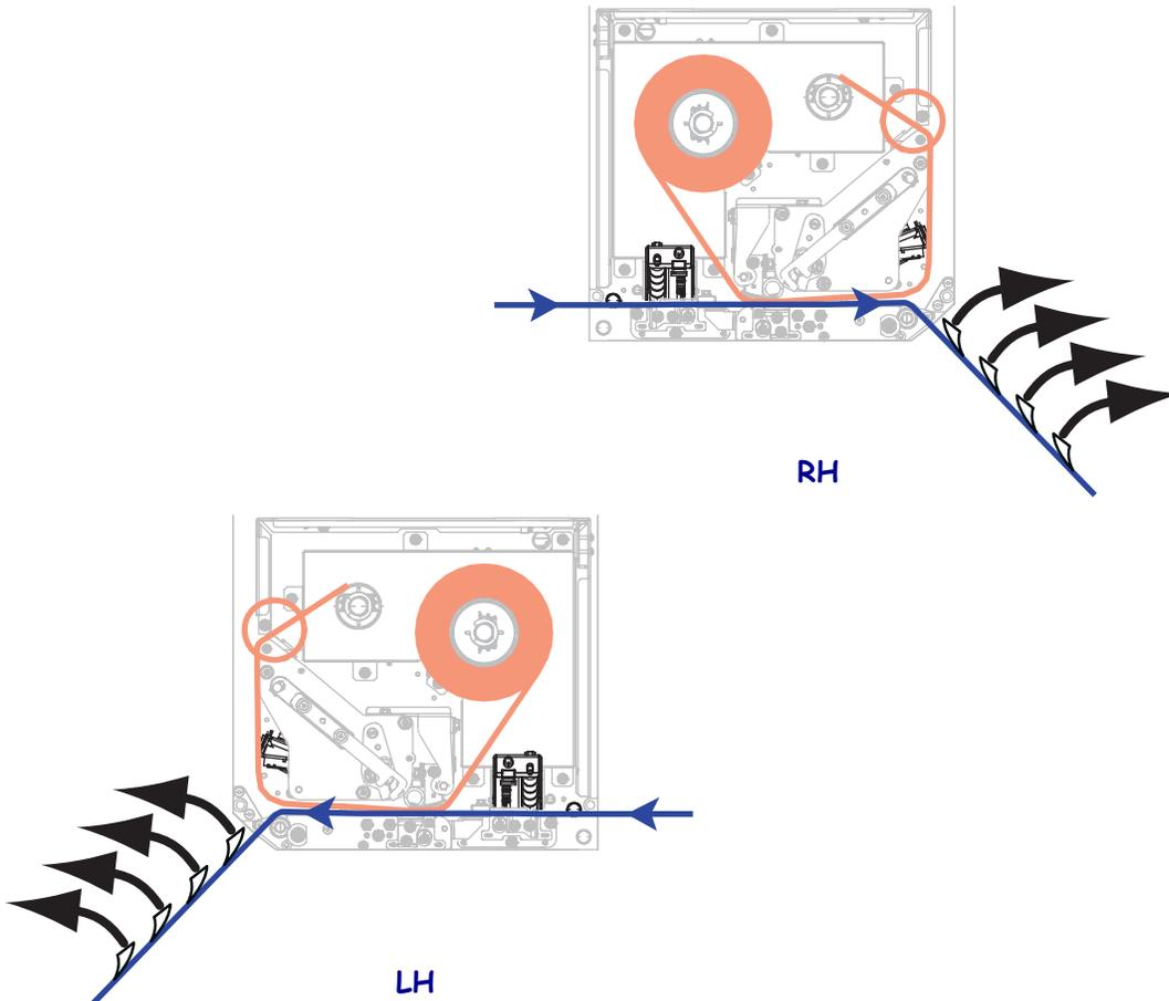
4. Pull the media back into the print engine so that only the liner is between the media sensors.
