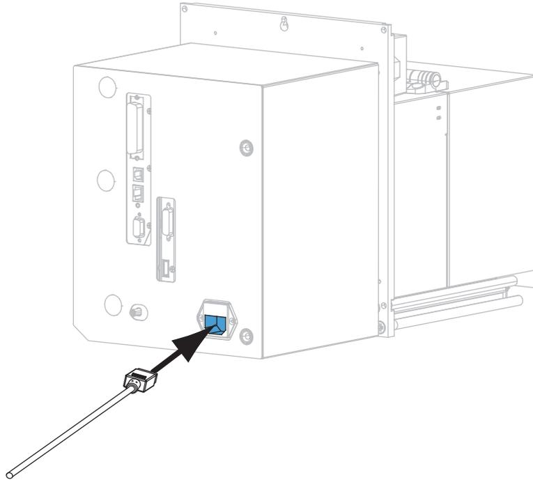
2. Plug the male end of the A/C power cord into an appropriate power outlet.
