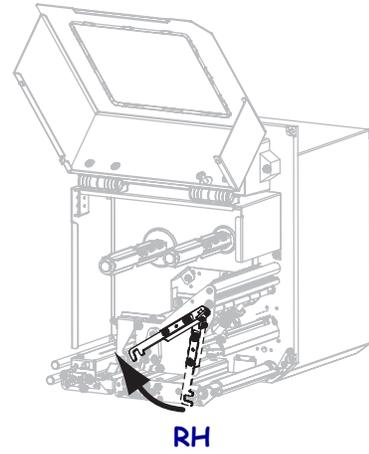
2. Position the ribbon roll with the loose end unrolling in the direction shown.
