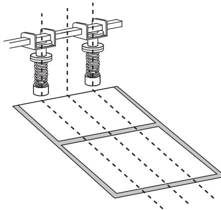
5. Tighten the locking nuts.
