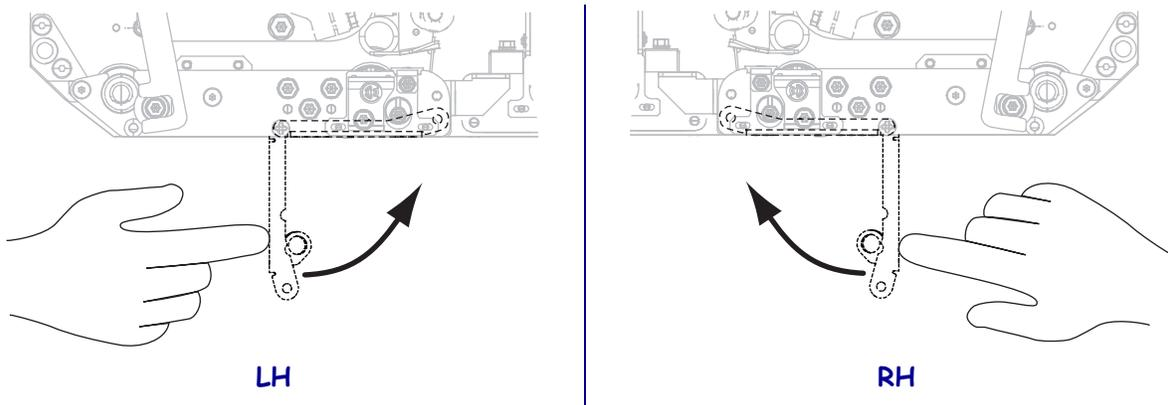
18. Thread the liner around the take-up spindle of the applicator (refer to the applicator's documentation for more information).
