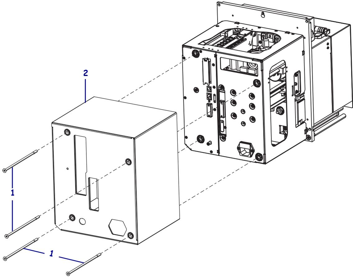
5. On the back of the applicator interface board, remove the two mounting screws (1) that secure the applicator interface board (2) to the back plane of the print engine.
