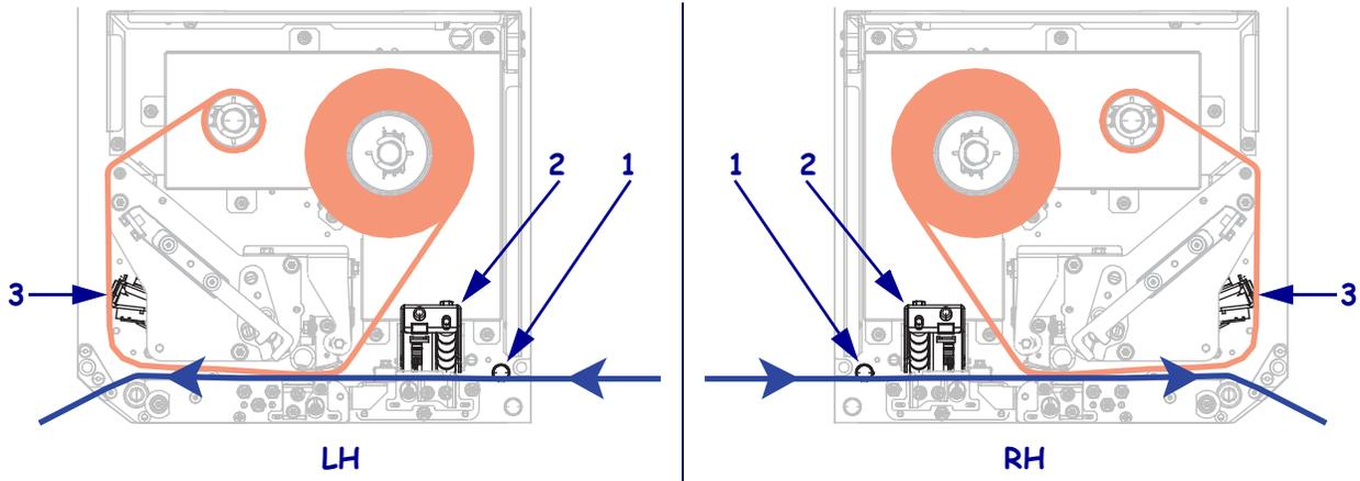
11. Extend approximately 30 in. (75 cm) of media past the peel bar. Remove and discard the labels from the liner on this exposed media.
