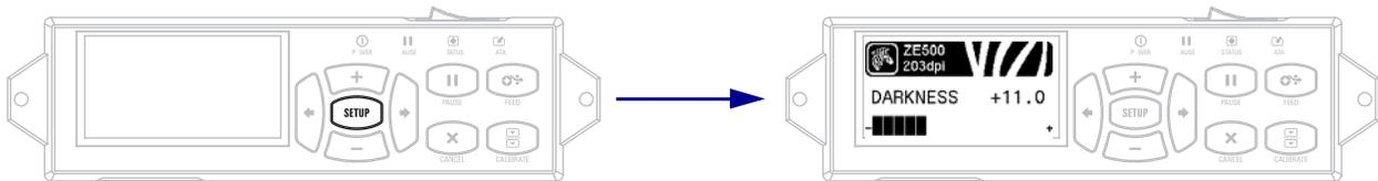
At the Idle Display (Figure 5), press **SETUP** to enter Setup Mode. The printer displays the first parameter.
