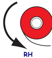
3. Place the roll of ribbon on the ribbon supply spindle. Push the roll back as far as it will go.
