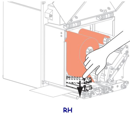
14. Rotate the printhead-release latch to the closed position.
