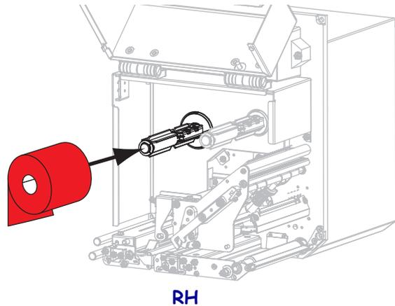
4. Place an empty ribbon core on the ribbon take-up spindle. Push the core back as far as it will go.
