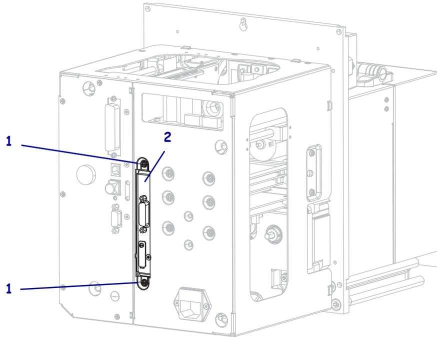
6. Locate the latch (1) on the side of the print engine.
