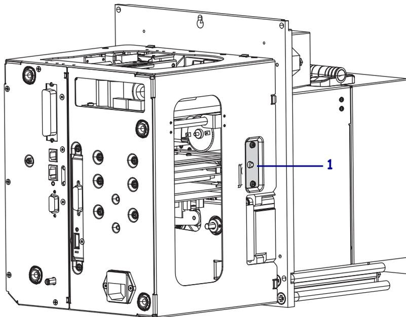
7. Press the latch, and then swing the electronics enclosure open.
