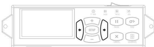
To scroll through the parameters, press the **LEFT ARROW** or the **RIGHT ARROW**.
