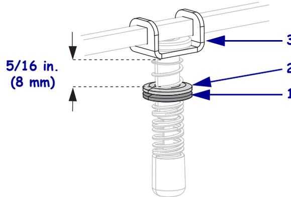
5. Move the adjusting nut until the print quality is acceptable. Use the lowest pressure that provides the desired print quality.
