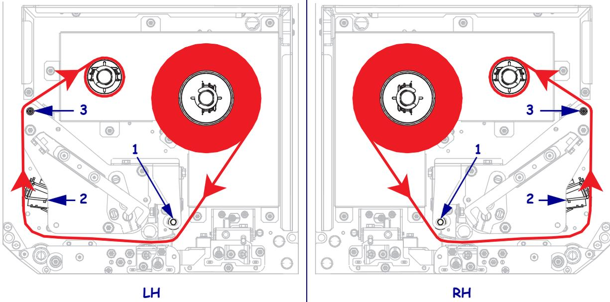
6. Wind the ribbon around the core on the ribbon take-up spindle.
