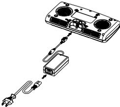
1. Connect the power cord to the adaptor for Quad Battery Charger/ Docking Cradle, and connect the adaptor for Quad Battery Charger/ Docking Cradle to the power connector of the Quad Docking Cradle.
