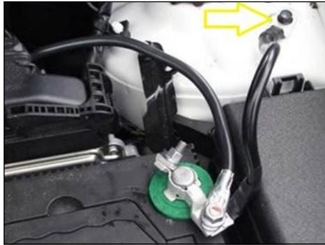
**Figure 4:** Heavy Wire Connecting to Chassis
