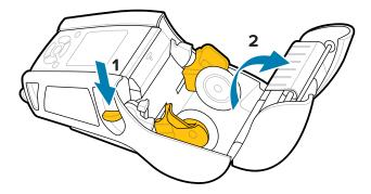
**2.** Pull the media supports apart and insert the roll of media between the supports in the orientation shown.
