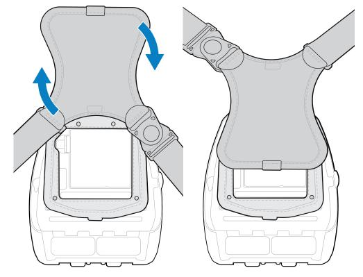
7. Snap the fasteners to secure (opposite side), and then rotate the waist strap 180°.
