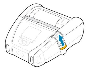
The peeler bail folds backward. The printer is now primed to remove labels from the roll automatically.
