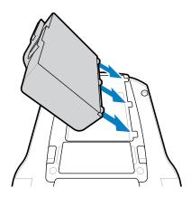
4. Rotate the battery into the compartment until it locks in place and is sitting flush with the printer.
