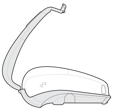
2. Rotate the top half of the hard case shell over the printer's top and snap shut.
