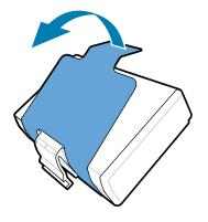
2. Peel back the tape insulator and remove it from the top of the battery pack. Discard upon removal.
