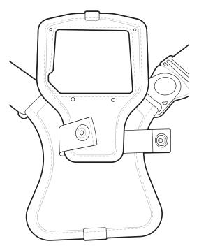
**2.** Unlock the male D swivel clip on the waist strap from the female D clip on the printer mount pad to remove it.
