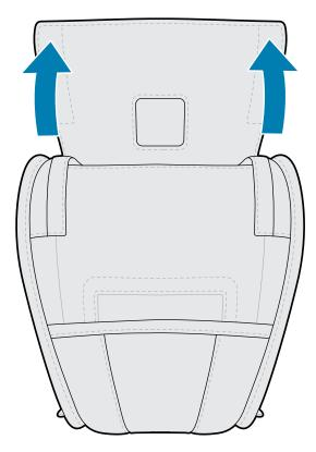
2. Slide the printer into the case so the LCD display is visible through the plastic window.
