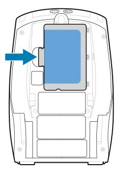
**3.** Rotate the pack away from the battery well, and then lift the battery up and out of the printer.
