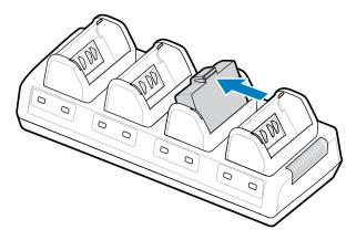
The amber indicator beneath the charging battery turns on when the battery is properly installed.
