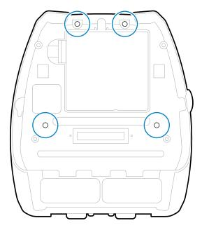
**4.** Use a 4mm hex driver on the two  $6-32 \times 0.375$  in. screws and two #6 washers to attach the mount pad to the top of the printer (circled).
