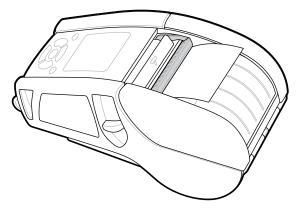
The peeler bail folds down. The printer is now primed to remove labels from the roll automatically.
