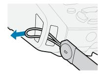
2. Loop the end of the strap back around the strap attachment point and secure it over the button.
