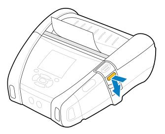
The peeler bail snaps forward to its original position and is now disengaged.
