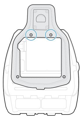
**5.** Attach the two  $6-32 \times 0.625$  in. screws and washers to the bottom of the mount pad (circled).
