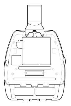
Figure 21 Metal Belt Clip with Hard Case
