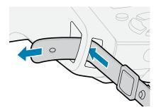
2. Insert the hole on the end of the strap over the metal fastener to secure it.
