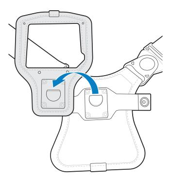
3. Align the holes on the mount pad with the mounting holes on the bottom of the printer (circled).
