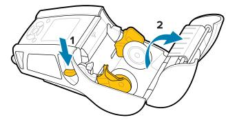
**3.** Pull the media supports apart and insert the roll of media between the supports in the orientation shown.
