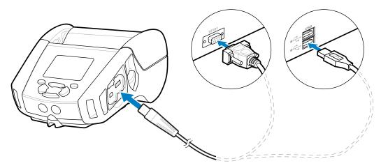
Zebra Designer Driver uses Windows drivers that support printing via Serial, USB, and the network. Mobile computers and other communication devices may require installing special drivers to use the USB connection. Go to <u>zebra.com/support</u> for further details.
