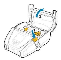
**3.** Pull the media supports apart and insert the roll of media between the supports in the orientation shown.
