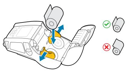
The supports secure the media in place and adjust to the width of the media. The media roll should be able to spin freely on the supports.
