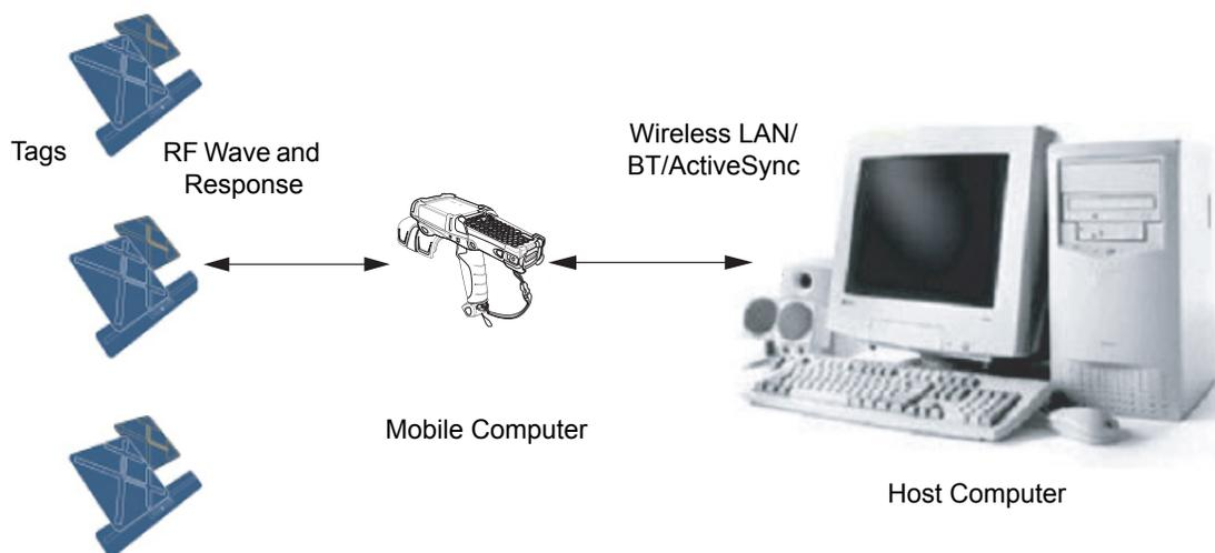
**Figure 1-1** RFID System Elements
