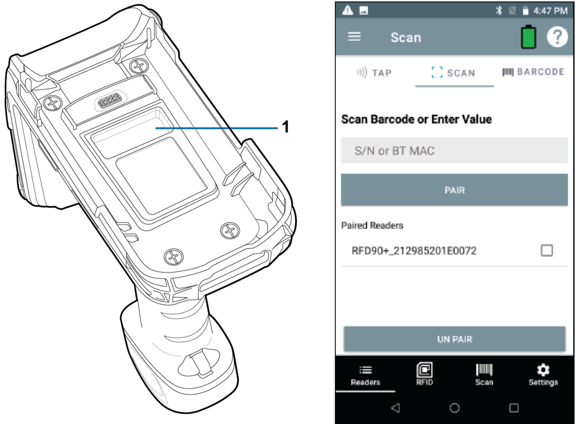
Figure 6 Scan 2D Barcode to Obtain MAC Address
