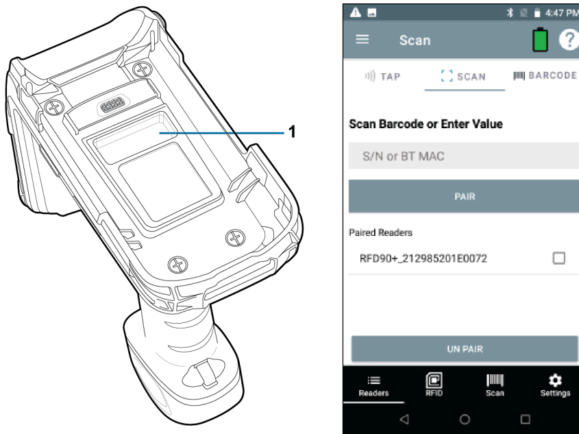
Figure 6 Scan 2D Barcode to Obtain MAC Address
