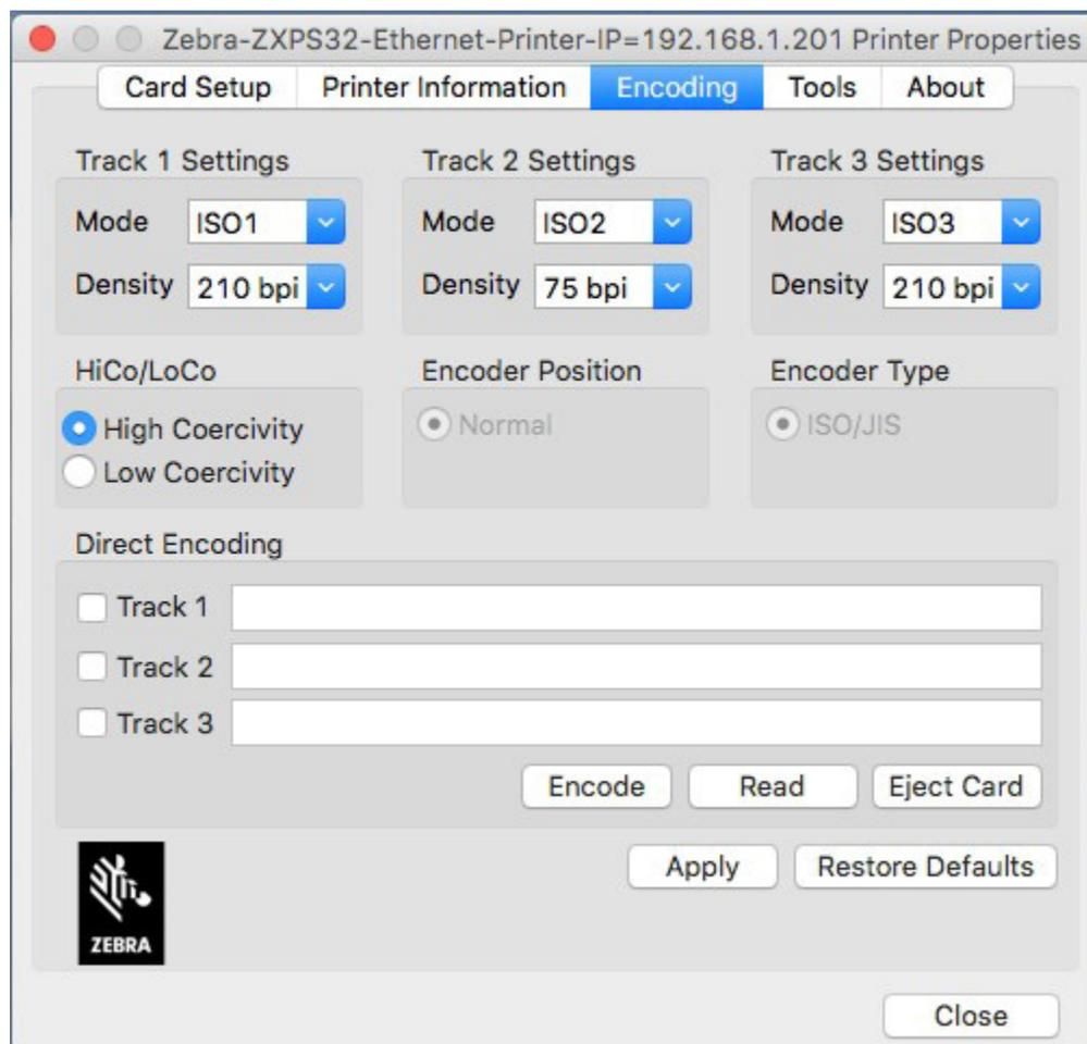
The Encoding tab is for setting Magnetic Encoder parameters. This feature is not enabled if the printer does not have the magnetic encoder option.
