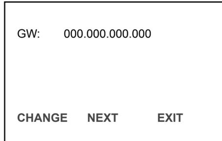
Use the **CHANGE** soft-key to change the selected digit. Each press of **CHANGE** increases the digit value by 1 with a roll-over to zero when necessary. The selected digit will flash. Use the **NEXT** soft-key to select the next digit in the sequence. Pressing **NEXT** when the last digit is selected will result in the first digit being selected.
