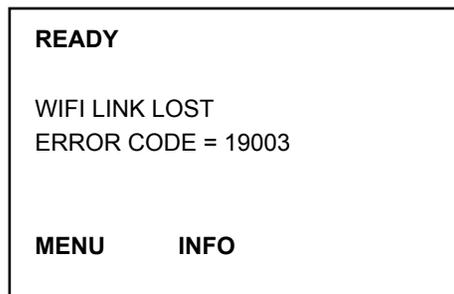
A wireless error is not considered an alarm condition, such as “Out of Cards”, so the display does not change to **ALARM**. The wireless error display is simply informative. In most cases communications with the printer will have been lost, so the wireless error condition will usually not be seen by a host.
