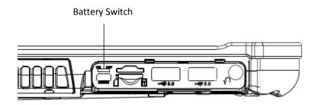
Battery Switch is ON when thrown toward the top side of the tablet.
