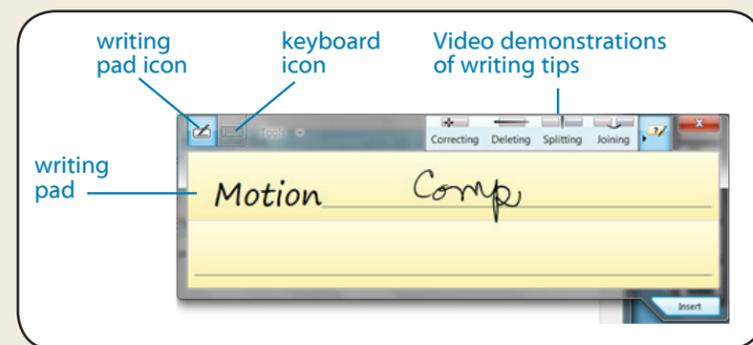
**TIP** Use the handwriting recognition application to train the C5m/F5m to recognize your handwriting style. To start the application, open Motion Dashboard, tap **Pen & Tablet**, tap **Pen & Input Devices**, and then tap the **Handwriting** tab.
