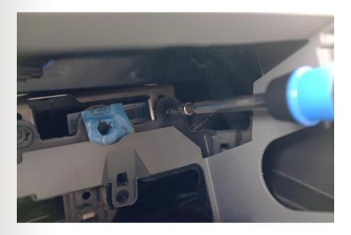
14) Remove the left hand chassis retaining bolt as shown.
