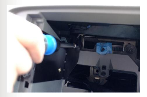
22) Note that the metal of the bracket is designed to bend and will be pulled in by the screw. Ensure that it is fully tightened.
