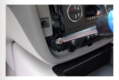
31) Refit the right hand retaining screw to the switch panel unit as shown.
