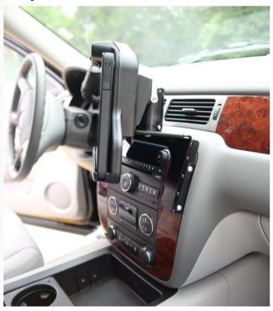
34) Fit the Docking Station / Tilt & Rotate Assembly to the front bracket as shown using the provided M8 fasteners.
