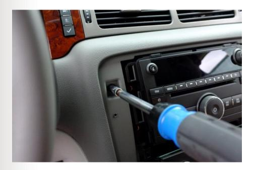
10) Remove the right hand fascia retaining screw as shown.
