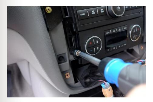
29) Refit the right hand retaining screw to the heater control unit as shown.
