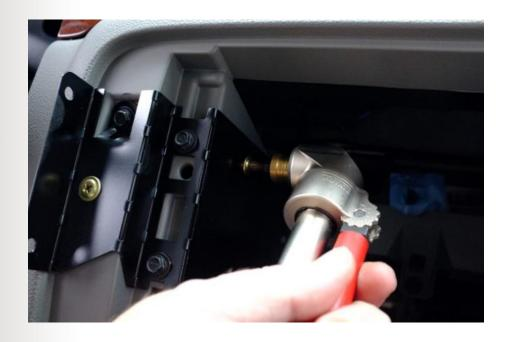
20) Fit one self tapping screws 039-02-0423 into the side as shown.
