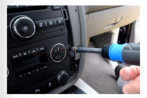
8) Remove both switch panel retaining screws. Only left hand screw is pictured.
