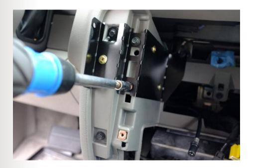
24) Remove the upper screw which was temporarily fitted in step 15.
