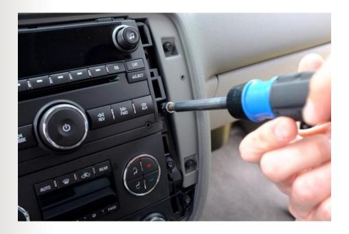
6) Remove the lower left radio retaining screw as shown.
