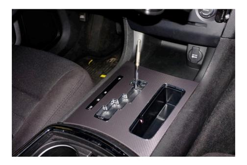
19) Slide the gear shift collar back on as shown.
