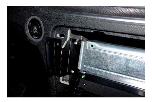
12) Refit using two of the screws removed in step 10.
