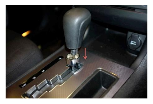
2) Remove the small clip retaining the gear shift knob as shown.
