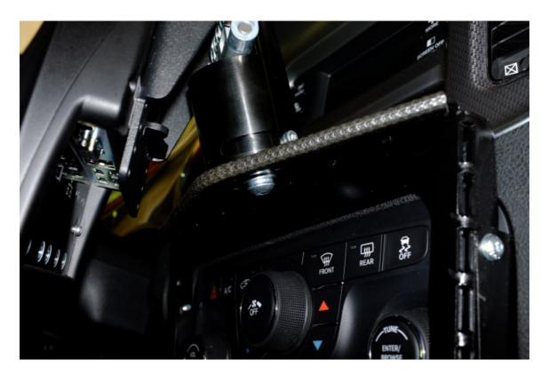
22) Fit the Docking Station / Tilt & Rotate Assembly to the front bracket as shown using the provided M8 fasteners.
