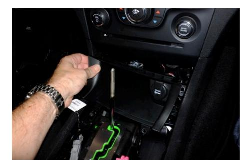
9) Remove the heater control panel as shown. Pulling firmly will release the retaining clips.
