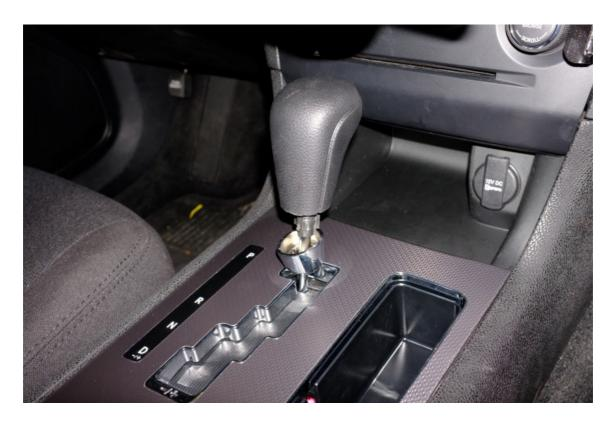
21) Refit the gear knob retaining clip and collar as shown.
