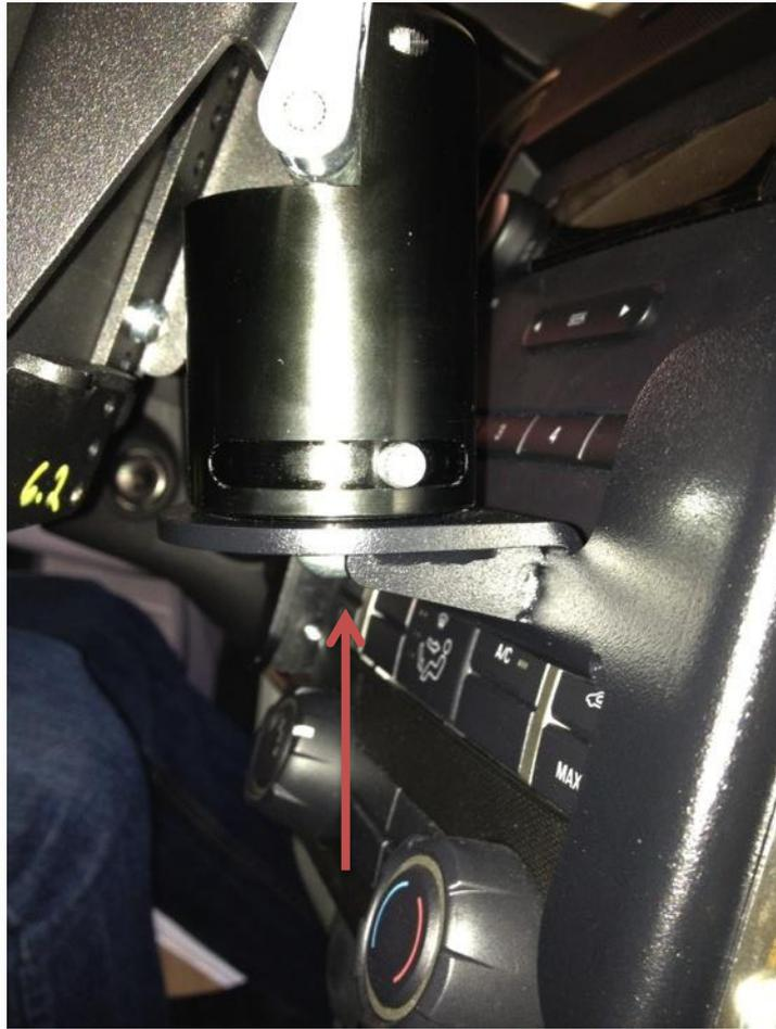
27) Fit the Docking Station / Tilt & Rotate Assembly to the front bracket as shown using the provided M8 fasteners.
