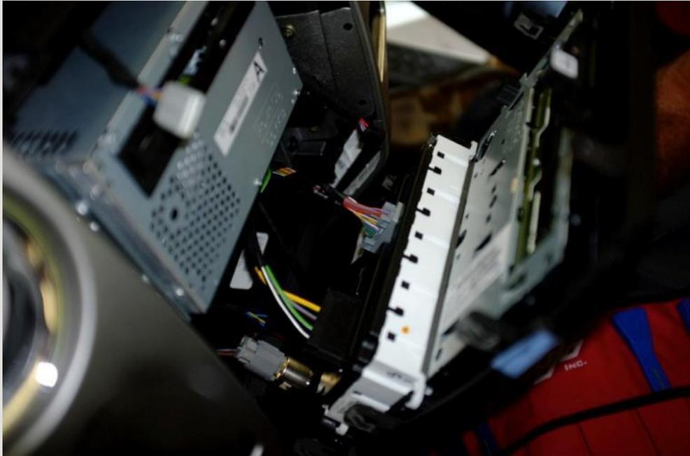
21) Refit the radio console as shown.
