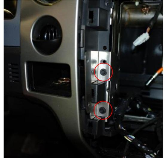
16) Fit two Lath Truss Screws TD504033 as shown being careful not to over-tighten.
