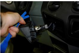
4) Disconnect the wiring loom by removing the plug.
