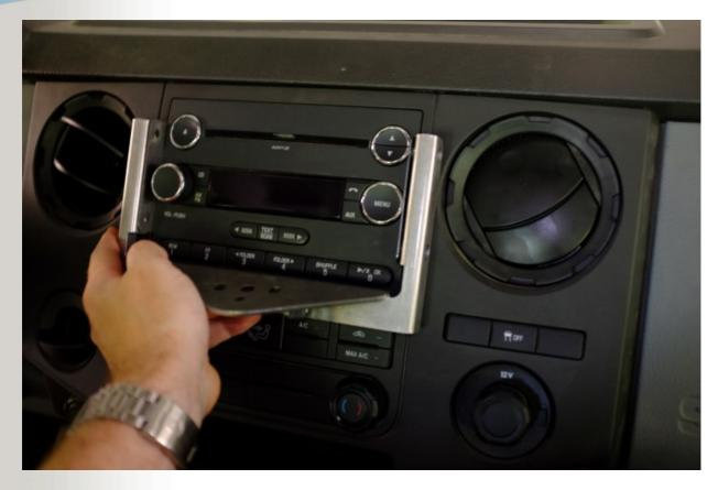
26) Fit the Front Plate 032-02-0312 as shown using two M5 Button head screws TD503712 and two Shakeproof Washers TD503481
