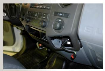
6) Pull the lower part of the dash panel forward to release the lower retaining clips. With a plastic trim panel removal tool, release the upper clips as shown.
