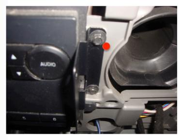
24) Using the bolts removed in step 22, fit the Left Hand Side Plate 032-02-0310 as shown. There is a small notch in the plate which must be towards the top as highlighted.
