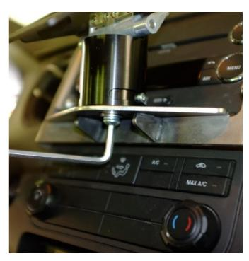
28) Fit the Docking Station / Tilt & Rotate Assembly to the front bracket as shown using the provided M8 fasteners.
