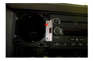
16) Fit the remaining M6 fasteners to the two holes as shown and fully tighten.
