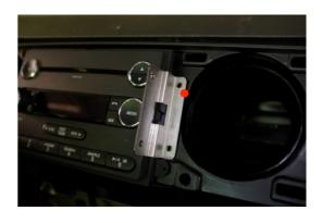
13) Fit M6 Button Head Screw TD504030, Shakeproof Washer TD504032 and Collar Nut TD504031 as shown.
