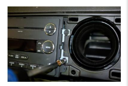
8) Remove the two left hand screws retaining the radio.
