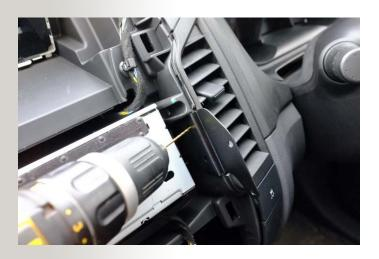
11) Drill two 2mm diameter pilot holes as shown and fit two self tapping screws as shown.
