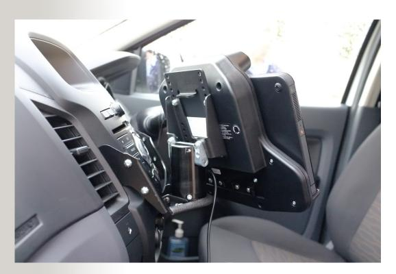
18) Fit the Docking Station / Tilt & Rotate Assembly to the front bracket as shown using the provided M8 fasteners.
