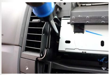
10) Fit the right hand side bracket (032-02-0297) as shown using the remaining screw removed in stage 8.
