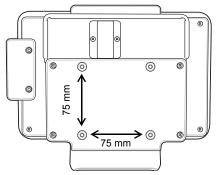
3. Secure the kiosk to the mounting surface using four M5 screws. The screw length may vary depending upon the mounting surface.
