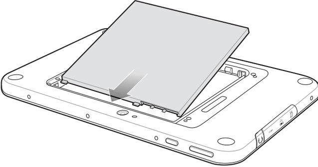
**CAUTION** Be aware of the orientation of the battery cover. Failure to replace the battery cover properly may damage the battery cover.
