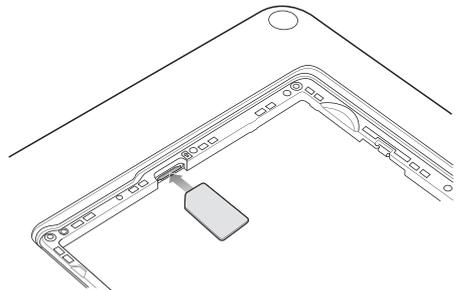
6. Push the micro SIM card in and ensure that it locks into place.
