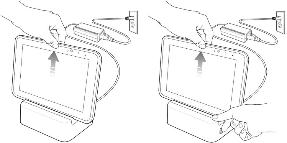
To remove the ET5X from either Communication Cradle, press the release button on the right side of the cradle and lift the ET5X. Use thumb to hold down the cradle.
