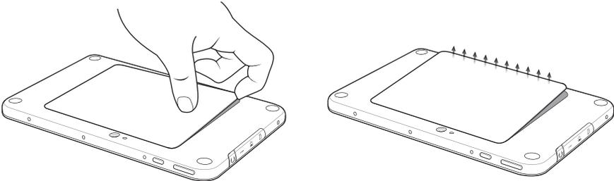
2. Carefully lift the battery cover off the ET5X.
