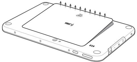
3. Carefully lift the battery cover off the ET55.
