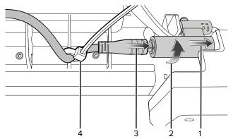
6. Route the cable around to the back of the dock as shown. A space is provided for the excess cable.
