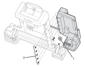
**4.** Plug the port expansion power cable into the power out port (1) on the dock.
