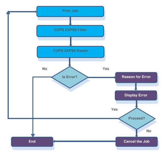
After collecting the Error Description, the component Error Display Mechanism displays the Error report for the user via a User Interface dialog. Then, it waits for a user response to that error report. Based on the response, either it continues the job or quits the current job. This error cycle continues until the termination of the current job in the printer. The previous flowchart describes how error handling works in CUPS.
