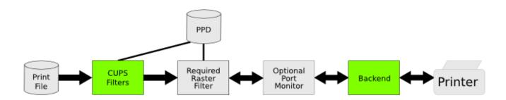
The raster filter converts CUPS raster data into a format the printer understands. The Zebra Filter will send the Zebra ZXP Series 3 printer commands along with the YMCK color buffer data to the backend.
