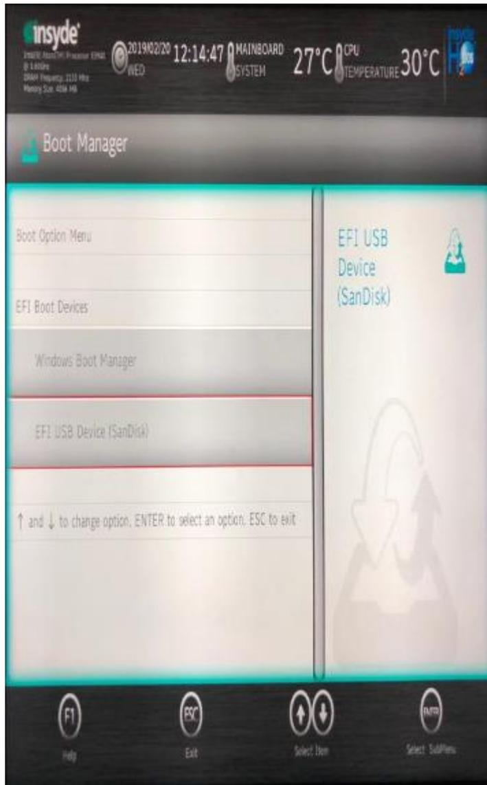
Select **“EFI USB Device”** using the **“down arrow”** from the keyboard and press ENTER. If Boot Manager does not display EFI USB Device (USB stick) confirm that the USB is formatted as FAT32 and bootmgr.efi file is visible in the USB stick. Re-seat the USB in the USB port and try again. If the problem persists see the [“Create a Bootable USB”](#) section at the end of this document.
