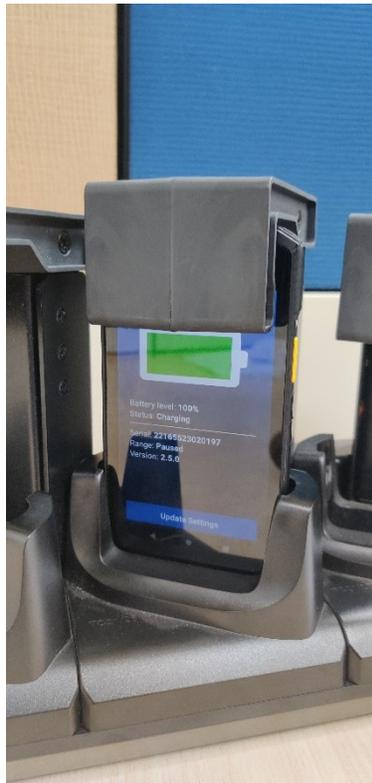
On “update settings” page select “scan to update” button as shown in the picture. Device starts scanner beam.
