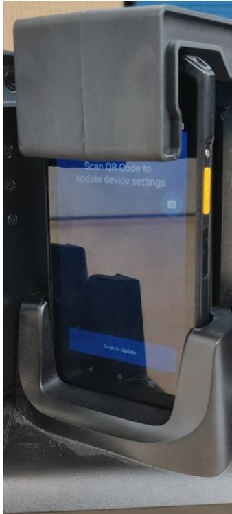
Place the QR code, printed on the paper, just above the device slot of cradle.
