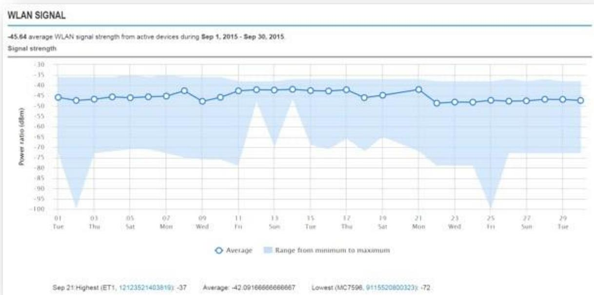
Figure B-58 Sample WLAN Signal Strength from SOTI
