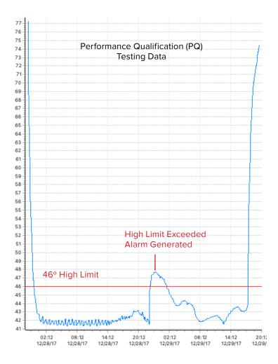
Temperature data for PQ testing was recorded by the M-300 sensor every 10 minutes over a 36+ hour period. Data was uploaded to the EDGEVue App to generate this graph. Note the 46° F High Limit (red line) was exceeded for approximately 2.5 hours.
