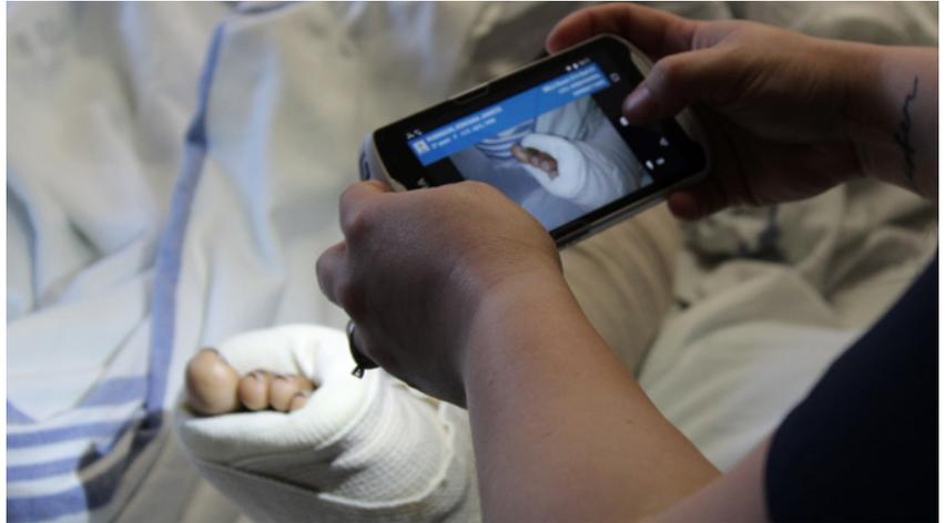
the TC51-HC mobile computer in just one minute, instead of the 10 minutes they used to spend disinfecting an isolation cart, not to mention the individual devices. In fact, the Zebra TC51-HC’s are built using Ingress Protection (IP) sealing that allows fast and safe disinfecting because it keeps liquid disinfectants from reaching the electronics.
