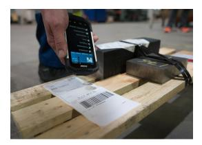
which assigns shipments to a certain vehicle and delivery route. Drivers receive pickup orders on their TC75s and use them to collect shipments. Each parcel is scanned with a TC75 whenever it is loaded onto or off a vehicle.
