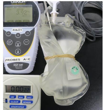
Test Group 3 External, Surface Temperature: Fluid-Filled Bag Wrapped Around Probe
