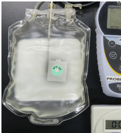
Test Group 1 Internal, Core Temperature: Probe into Center of Fluid-Filled Bag
