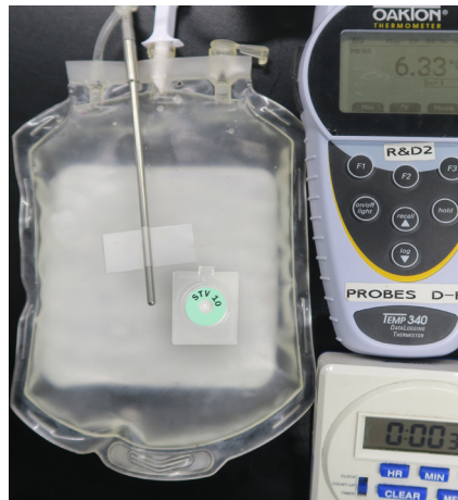
Test Group 2 External, Surface Temperature: Probe Taped to Surface of Fluid-Filled Bag
